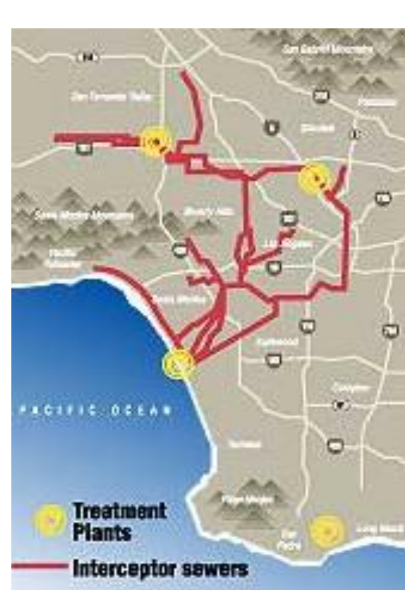
(left) The City's main sewer network is highlighted in red. These interceptor sewers convey wastewater flows to the four treatment plants (in yellow).
