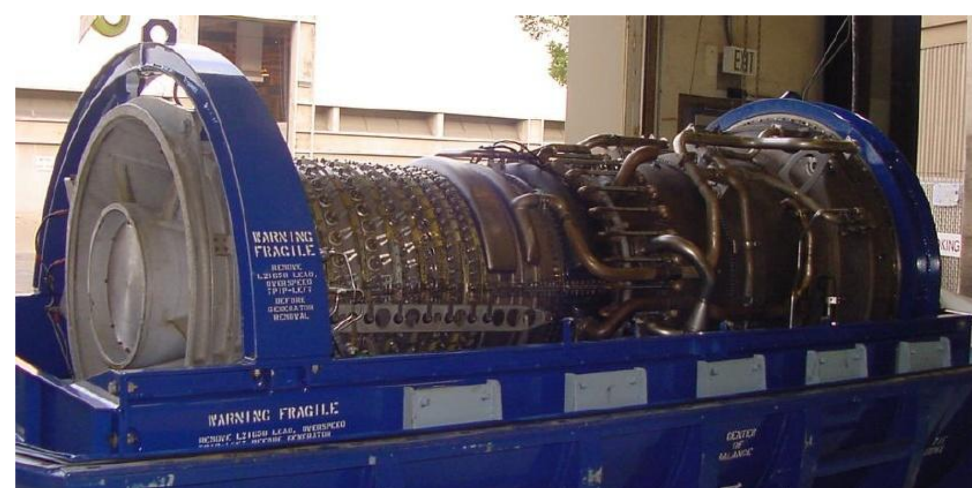
Inspecting the LM2500 requires disassembling it piece-by-piece.
