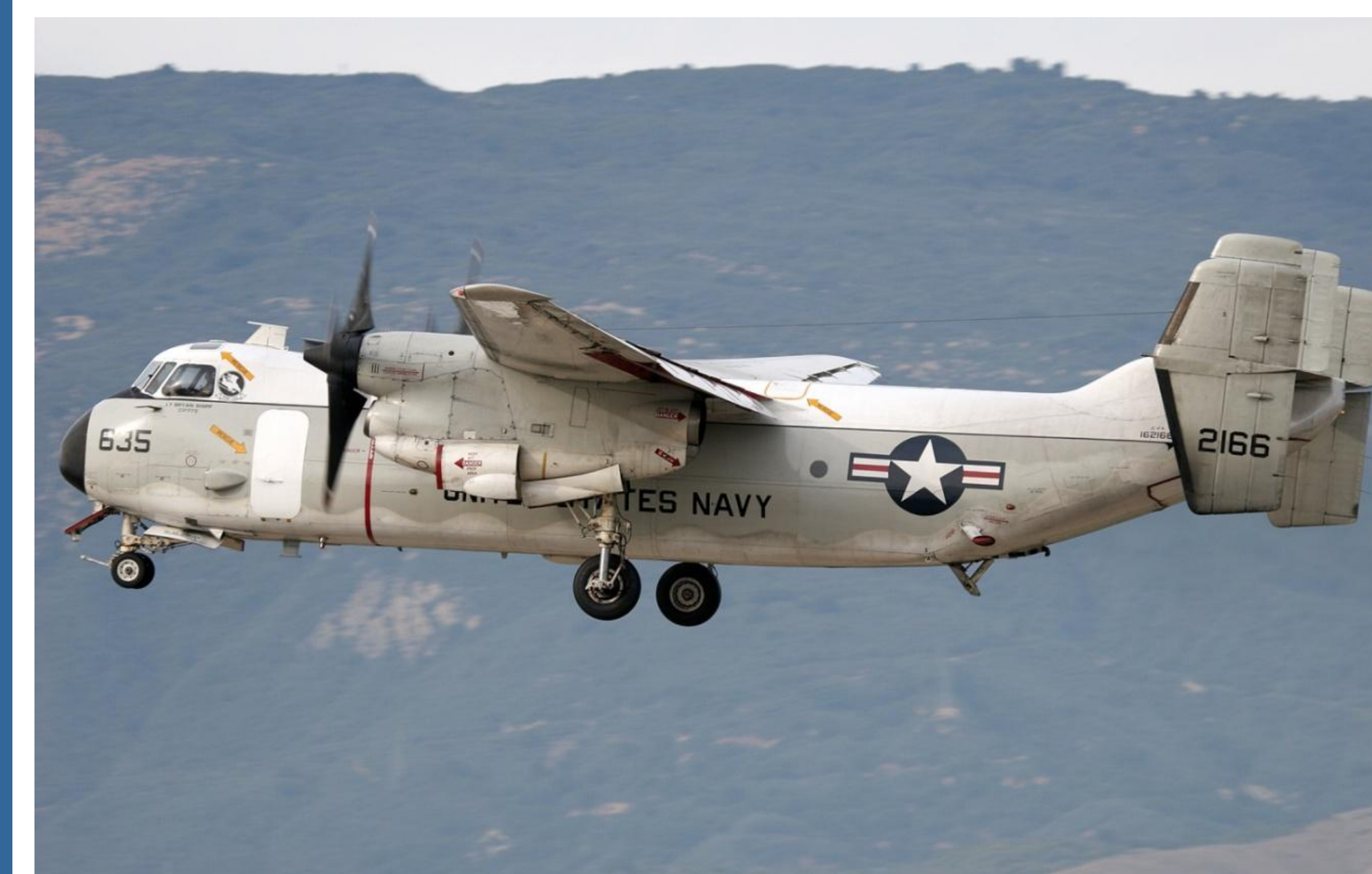
The upper longeron area is the main structural concern of the aircraft
