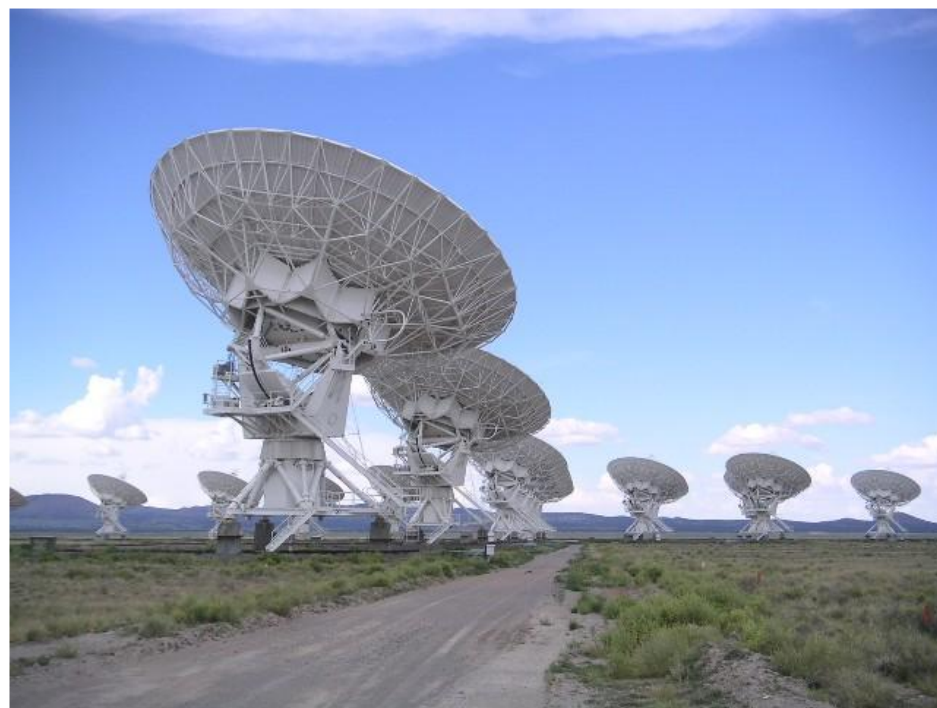
Large parabolic dish antennas are used to study celestial objects such as Pulsars at radio frequencies. Pictured above is a Very Large Array (VLA) interferometer in New Mexico.
