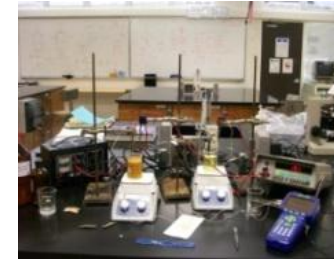
Figure 1. Electrolytic cell consisting of an Iron plating solution followed by an antimony solution.
