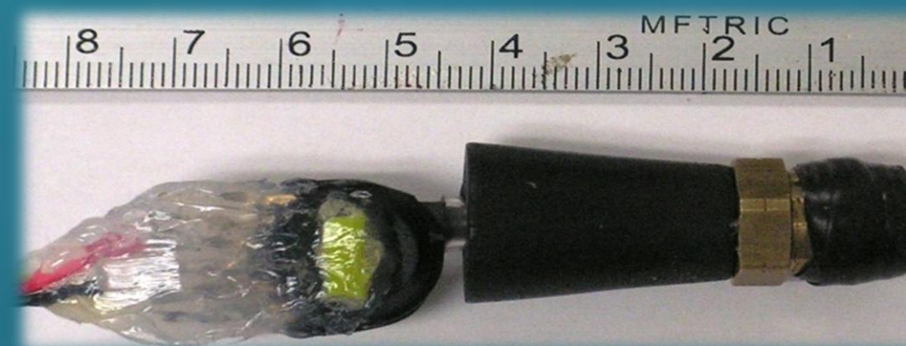
Franks' pressure sensor (Frankenstein pressure sensor).
