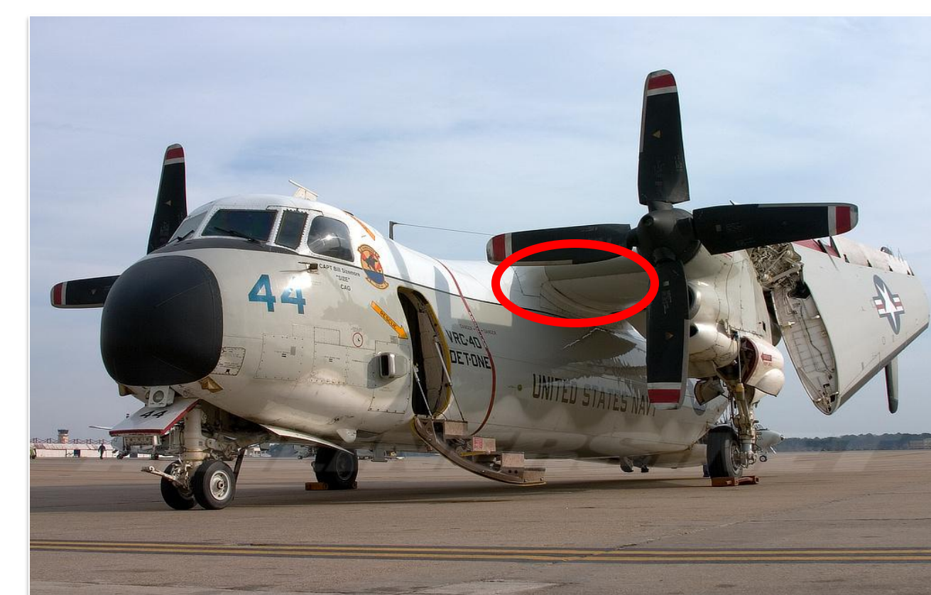
The red oval on the figure depicts the upper longeron area of the C-2A. This is also the area where the wings are attached to lugs. While in the air, the aircraft's own weight is being sustained by the lugs and hence the high stress.
