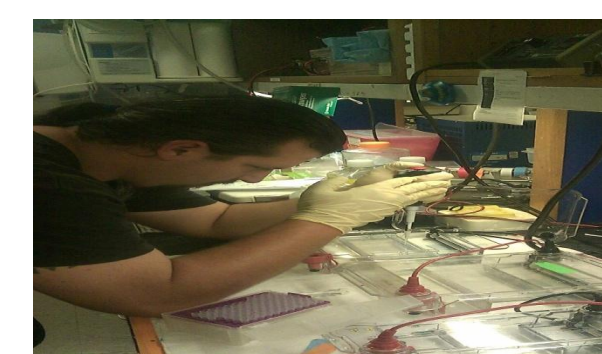
Fig 3: Steve Almos loading amplified DNA product into an agarose gel for electrophoresis.
