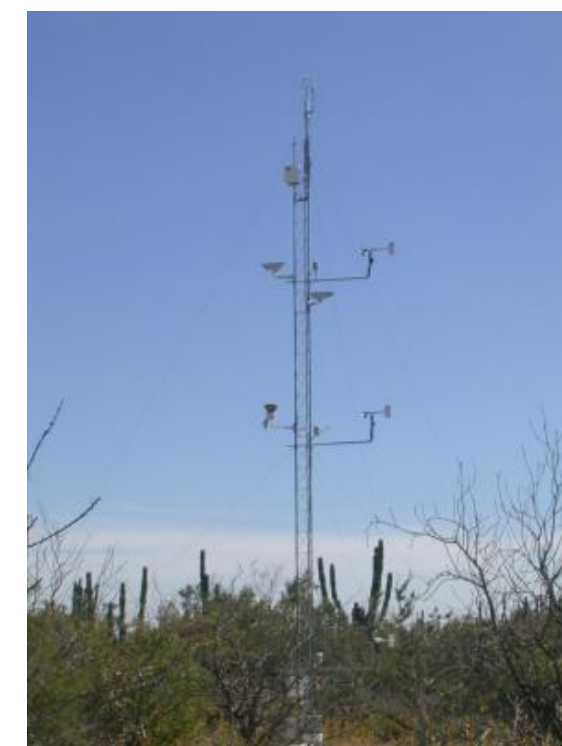
Fig. 2 This is the top of the Eddy Covariance system, which sits the Infrared Gas Analyser (IRGA) that detects CO 2 and H 2 O gas, and a Sonic Anemometer to record vertical turbulent flux.
