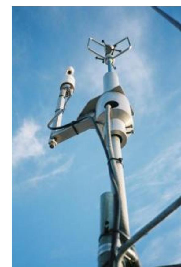
Fig. 2 This is the top of the Eddy Covariance system, which sits the Infrared Gas Analyser (IRGA) that detects CO 2 and H 2 O gas, and a Sonic Anemometer to record vertical turbulent flux.
