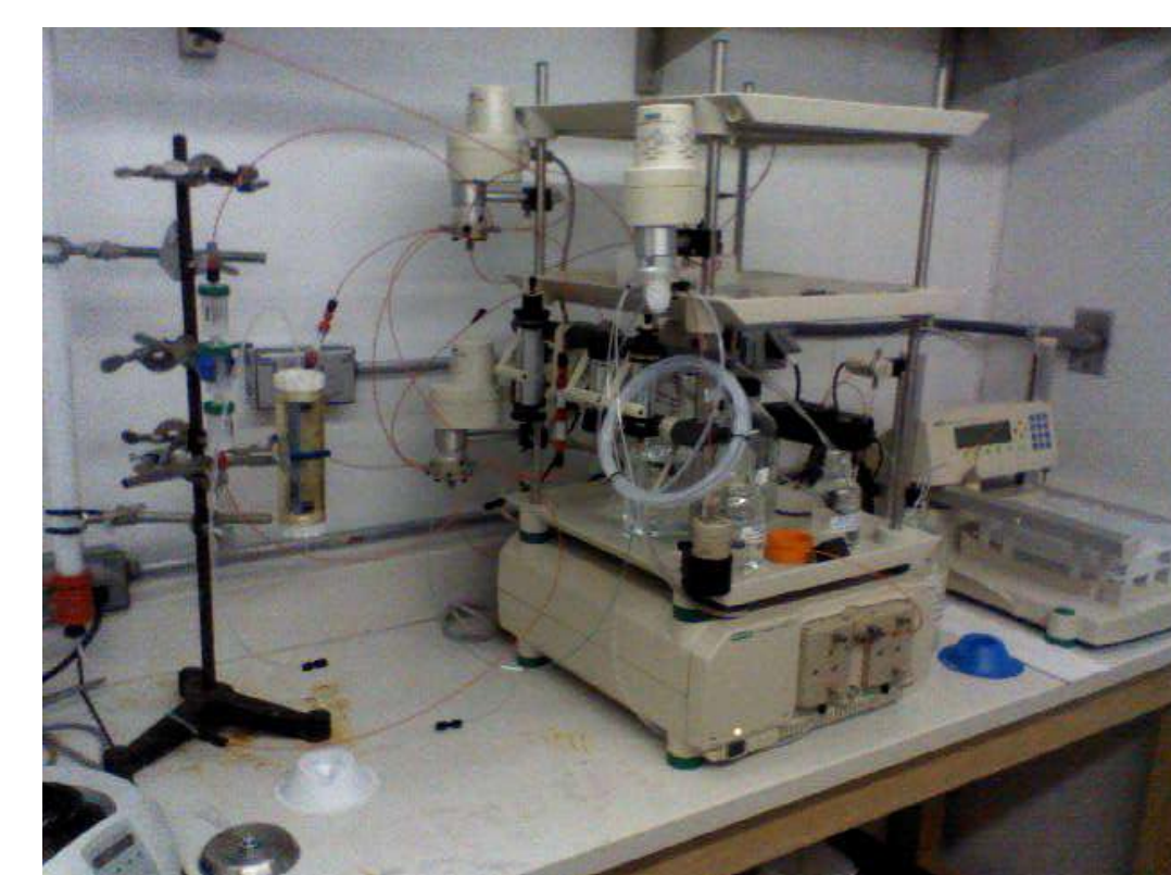
Fast Protein Liquid Chromatography (FPLC) was used to purify the enzymes using affinity (Nickel column) and gel filtration (desalting column) chromatography.
