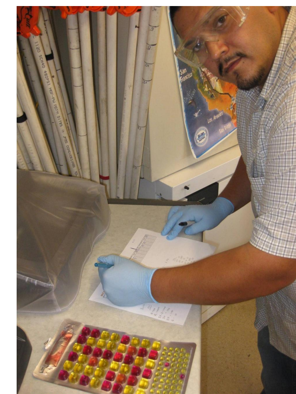
Left. Alberto Vasquez at San Diego Coastkeeper counting E.Coli positive water samples (red wells).
