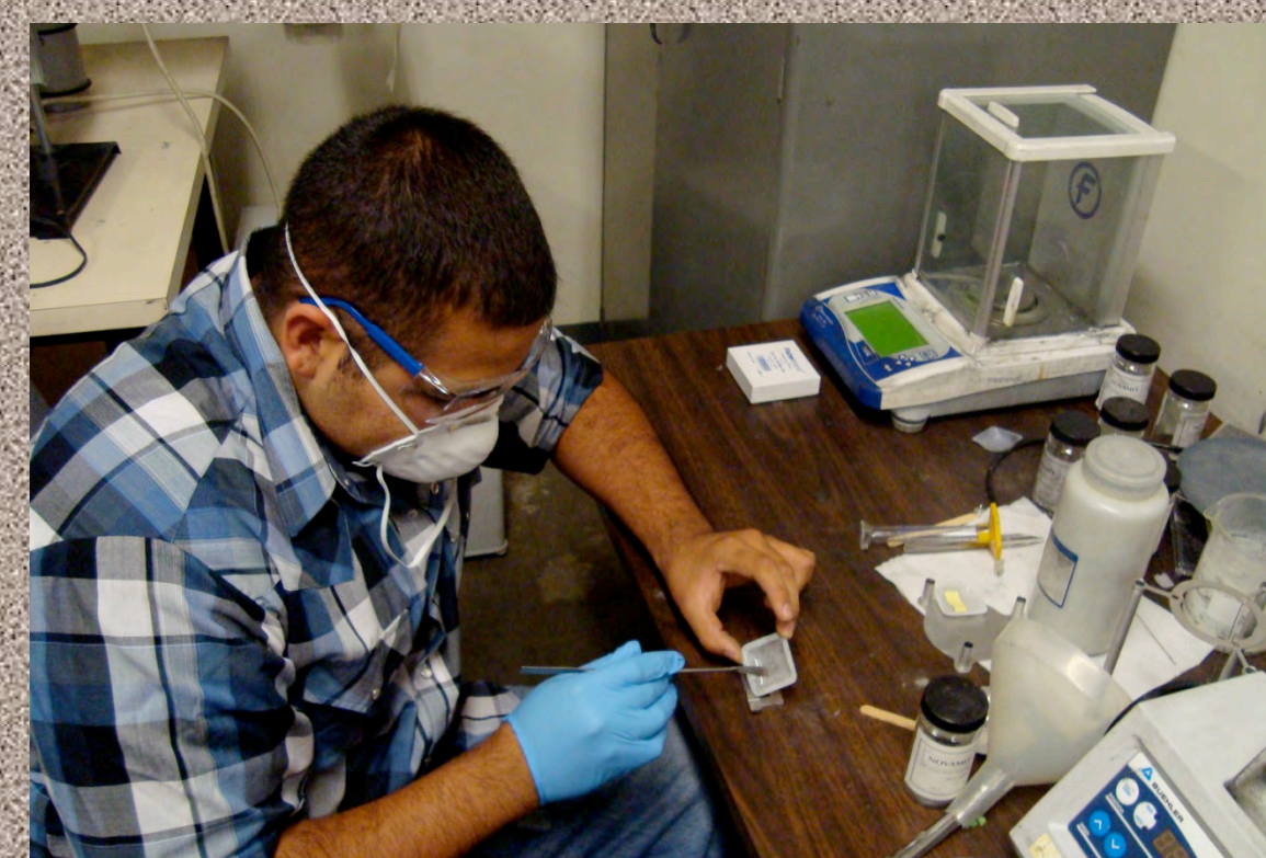
Ismael working in the laboratory — measuring and preparing a sample by filling the specimen with 316 stainless steel powder (left).
