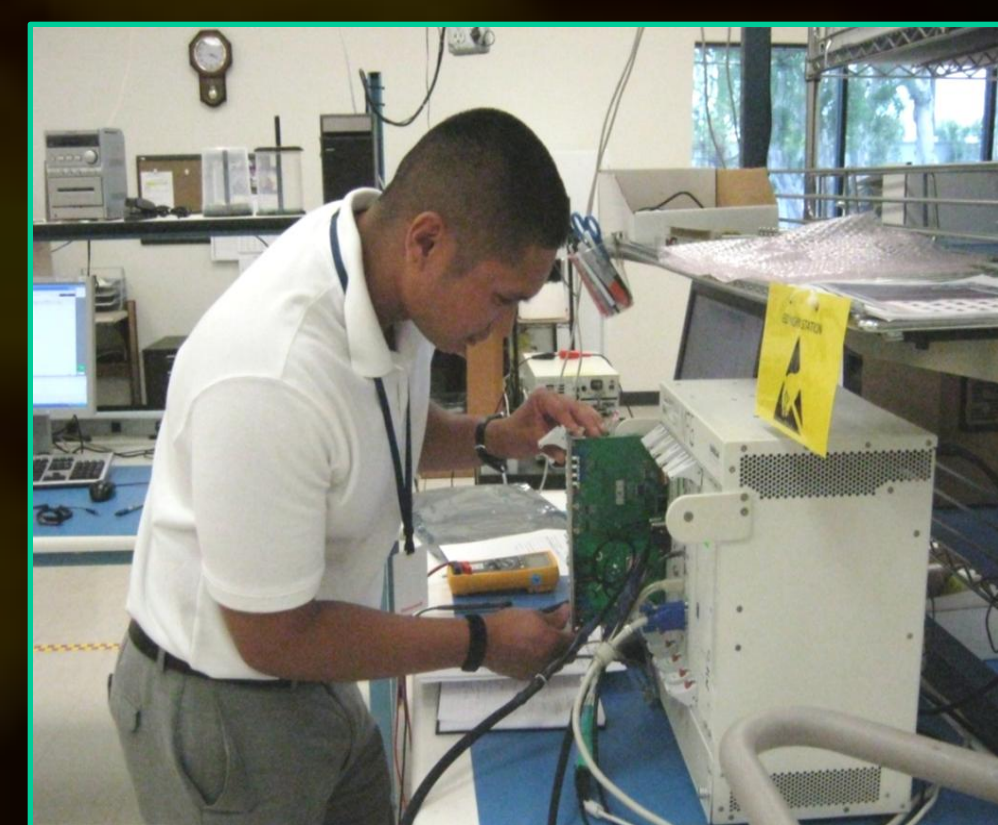
Russell Arroyo inserting the trigger board into the card cage to be programmed.
