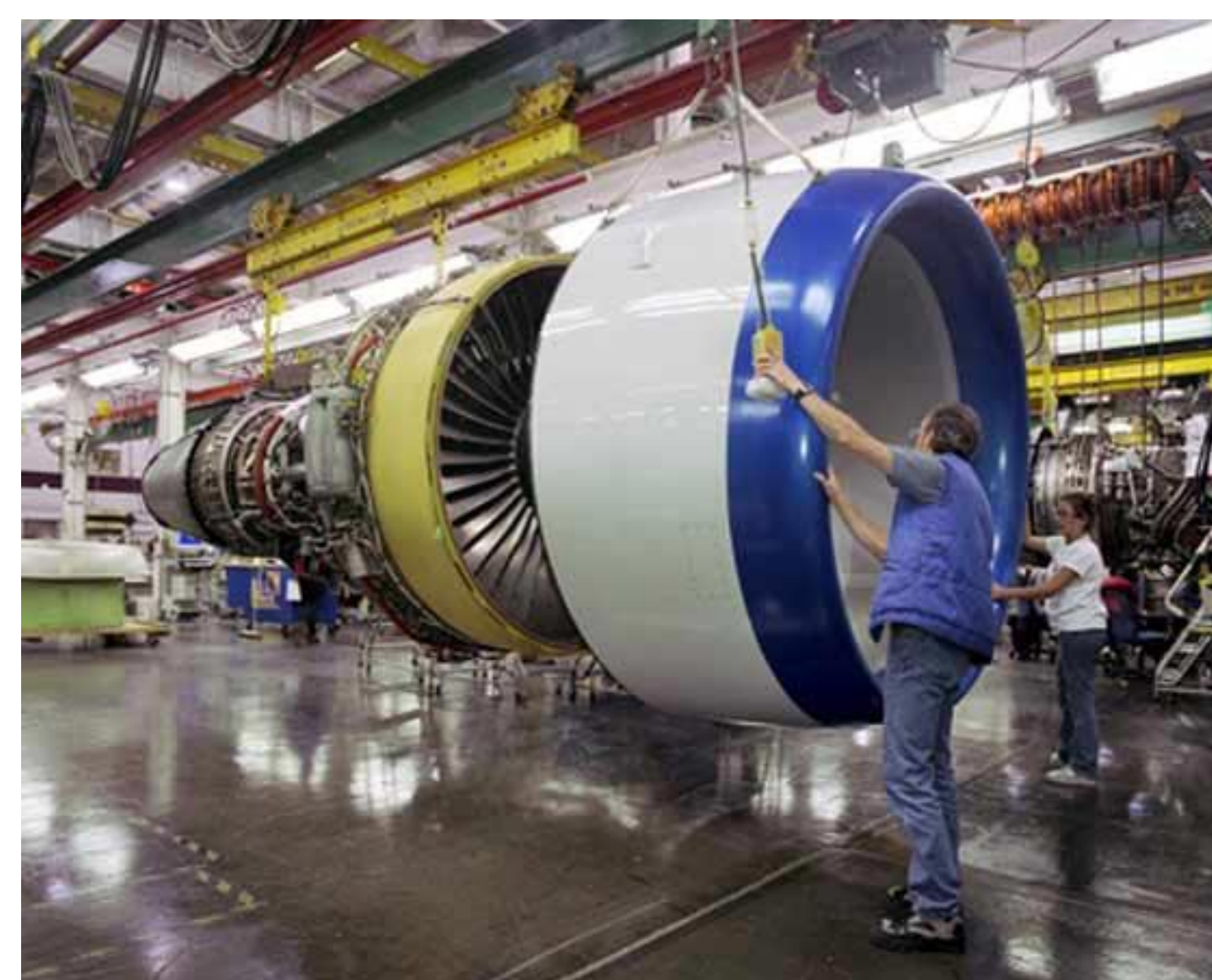
Workers assembling a nacelle air inlet lip and fan cowl onto a jet turbine.
