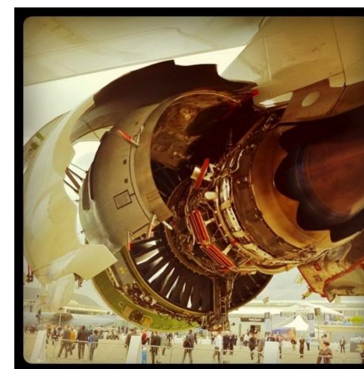
A nacelle and pylon mounted on an aircraft's wing with open compartments. Equipment Engineers are in charge of all the equipment mounted both around the engine and on the nacelle.
