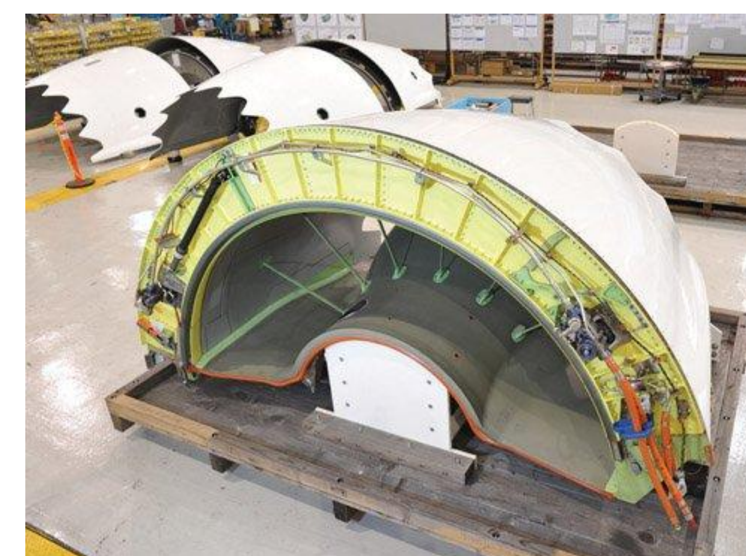
Part of the reverse thrusters cowl and air duct assembly. The picture also shows some of the equipment that helps the nacelle system function properly and safely.
