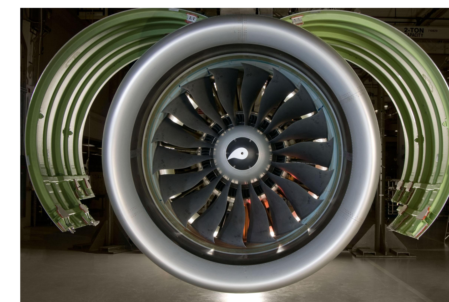
Design and Equipment engineers (as well as other Stress, Quality, Safety, and Systems engineers) work together to meet production goals towards developing a final product for their customer. Above is a front view of an assembled nacelle and turbine system with its cowl compartment doors opened.
